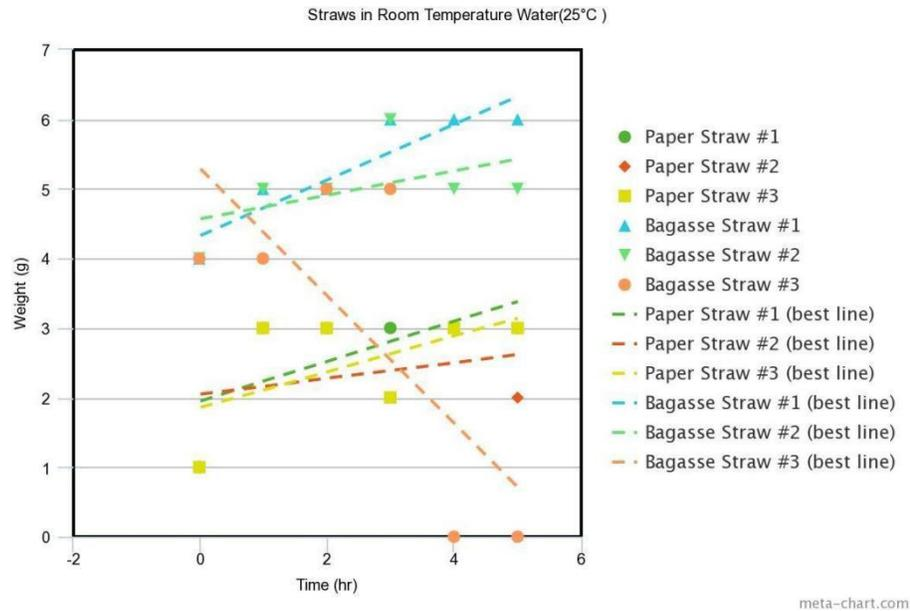
**Fig.I.1.** Weight gained by the bagasse straw & paper straw at room temperature water (25°C). Horizontal line x = time in hours (hr); vertical line y = weight in grams (g).
