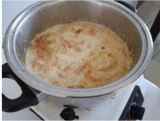
Fig 1. Cooking of bagasse in caustic soda to achieve pulp.
