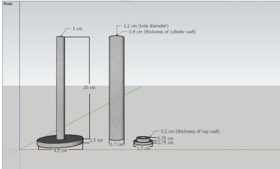
Fig 1. Metal Mold with measurements designed with the program SketchUp (2018).
