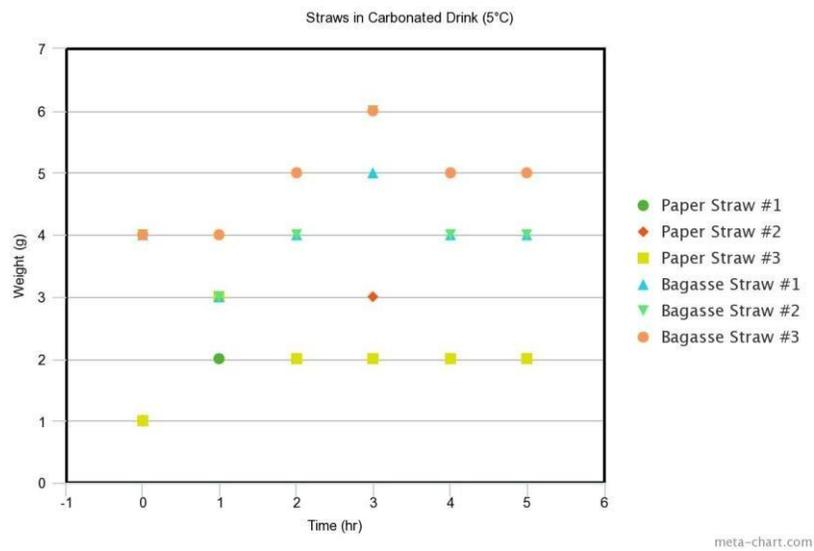
Fig. 4. Raw Scatter Plot of Straws in a Carbonated Drink (5°C).
