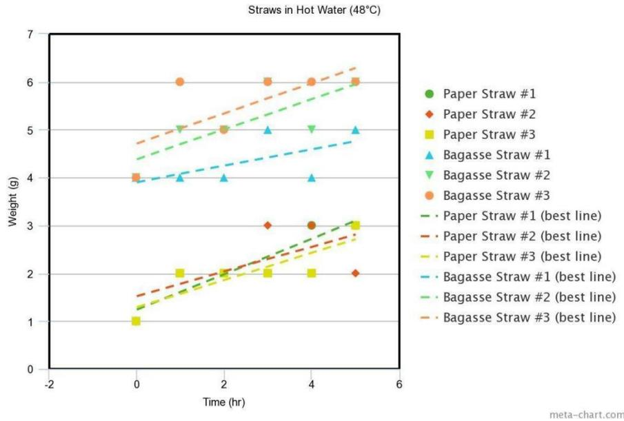
**Fig.I.2.** Weight gained by the bagasse straw & paper straw in hot water (48°C).
