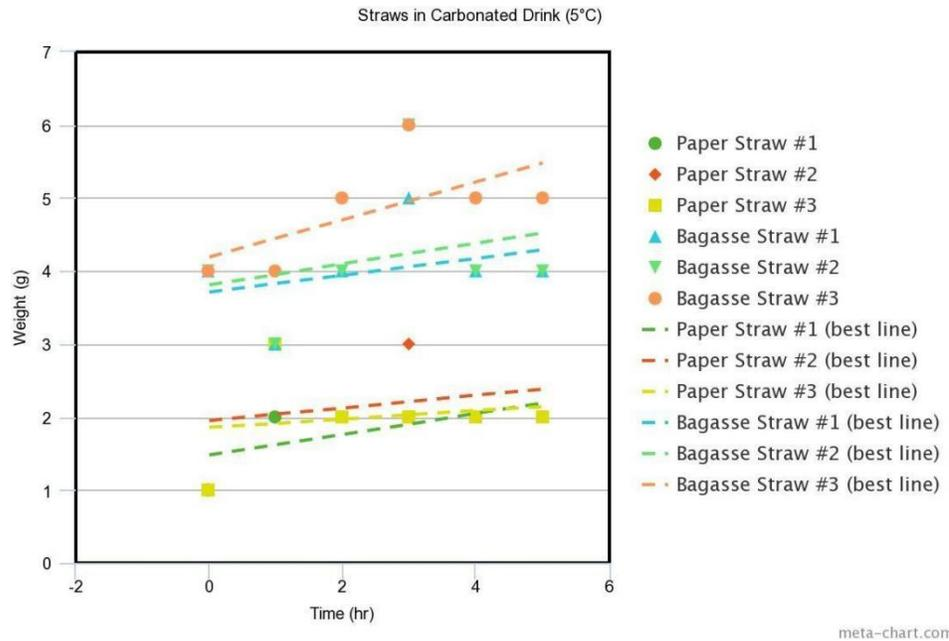
**Fig.I.3.** Weight gained by the bagasse straw & paper straw in a carbonated drink (5°C).
