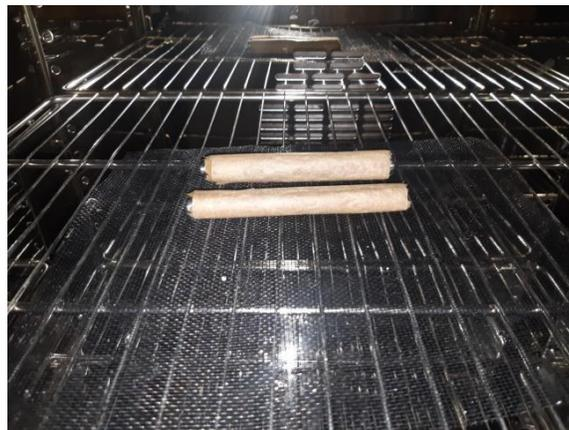
Fig 2. Straw-molded bagasse pulp in the drying oven.
